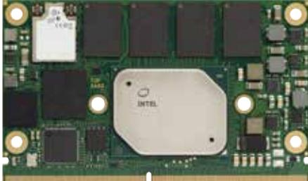
The congatec SMARC 2.0 module is equipped with Intel Atom, Celeron and Pentium processors (code name Apollo Lake) and suitable for outdoor use in smart city applications.
